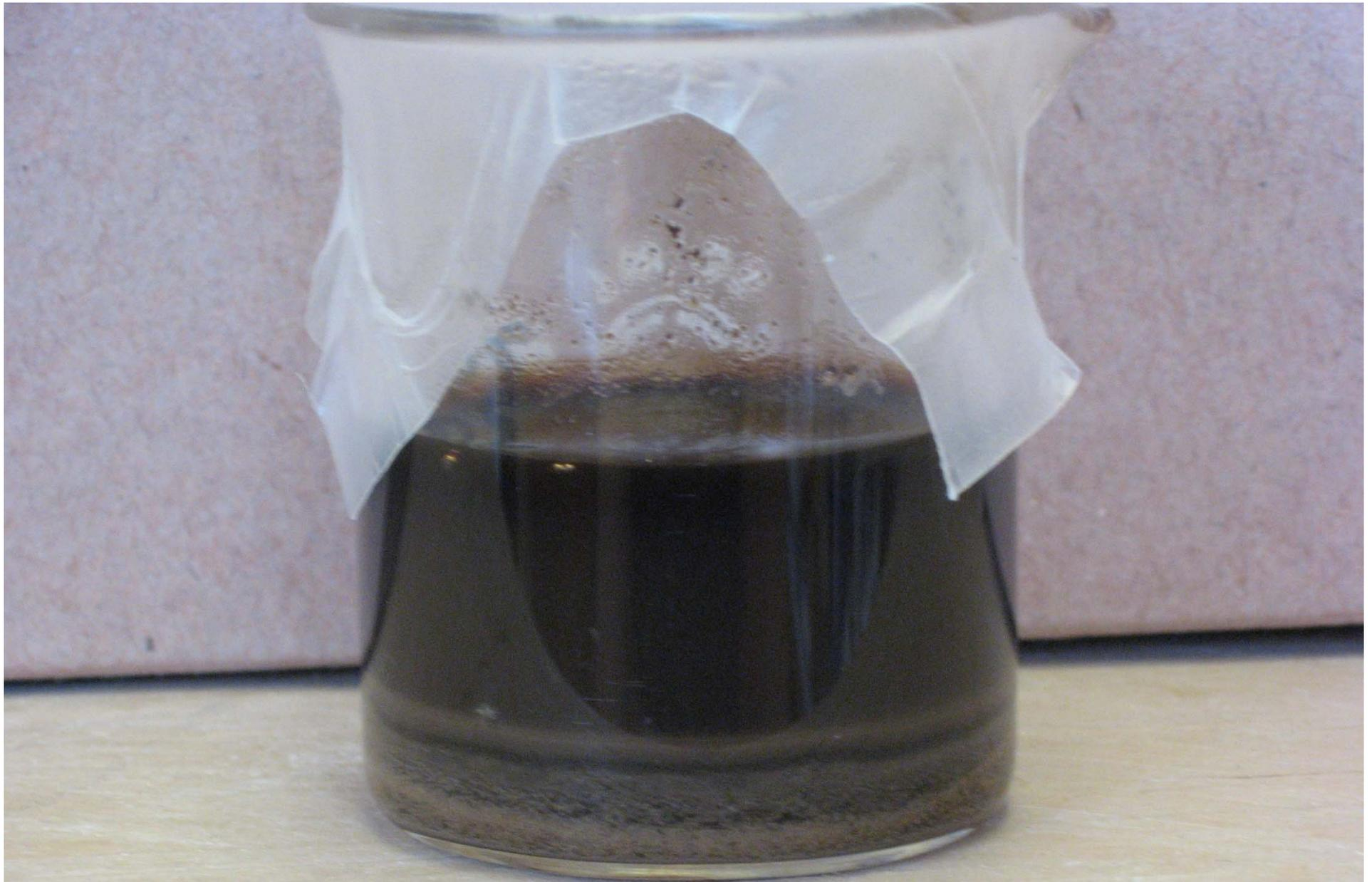
Dispersion of 1-cm core segments in 1% sodium polymetaphosphate and mechanical agitation, here allowed to settle showing bands of sand, silt and suspended clay, for particle size determination by laser scattering—after removal of pea gravel by sieving.
