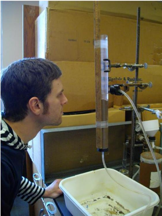
**Figure 2: Measuring Hydraulic Conductivity**
