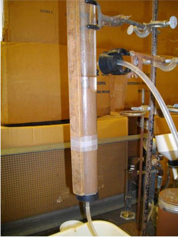
**Figure 1: Permeameter Setup**
