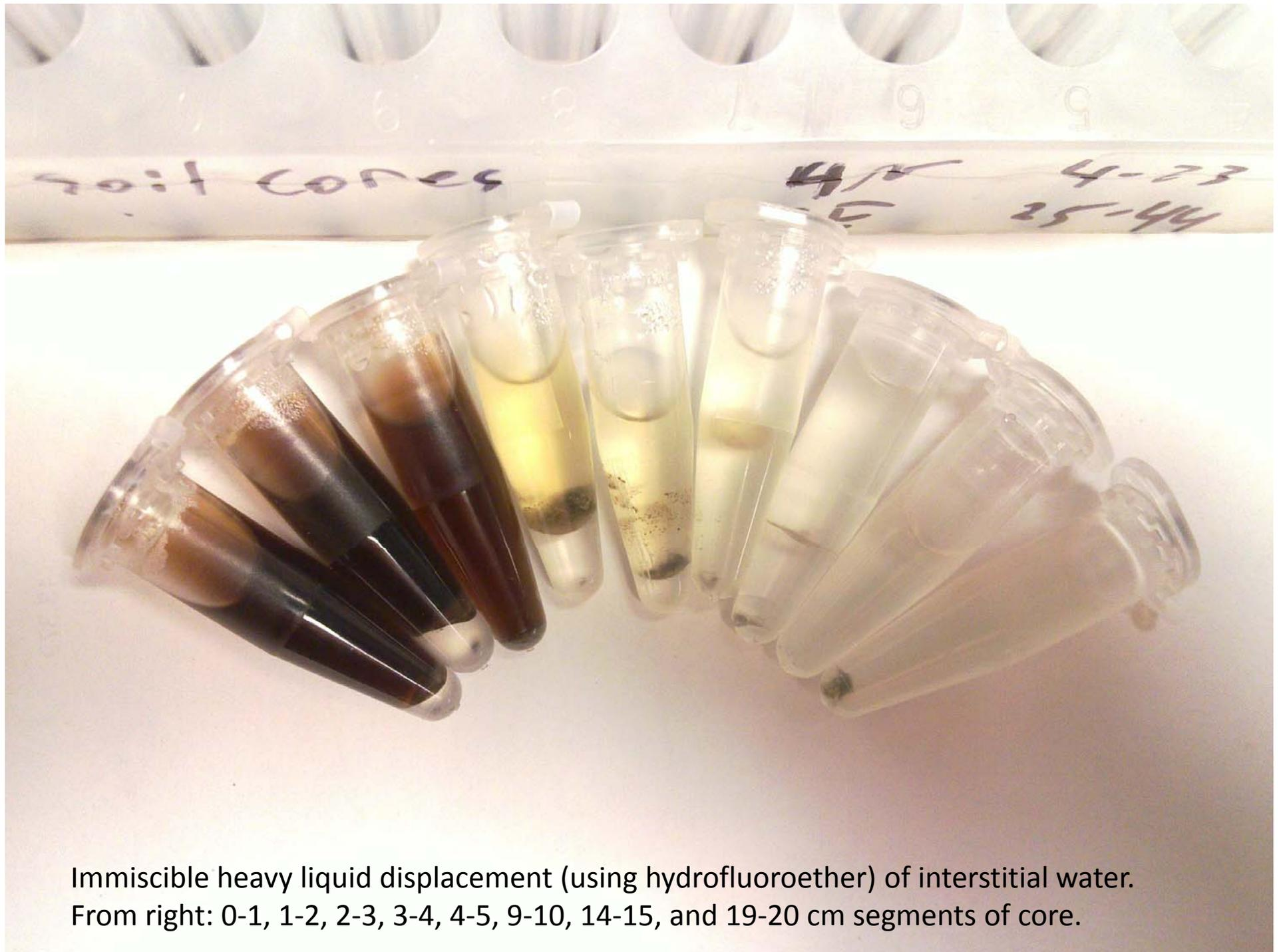
Immiscible heavy liquid displacement (using hydrofluoroether) of interstitial water.
