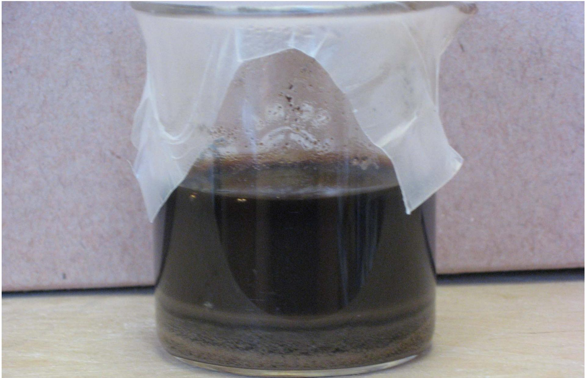
Dispersion of 1-cm core segments in 1% sodium polyphosphate and mechanical agitation, here allowed to settle showing bands of sand, silt and suspended clay, for particle size determination by laser scattering—after removal of pea gravel by sieving.
