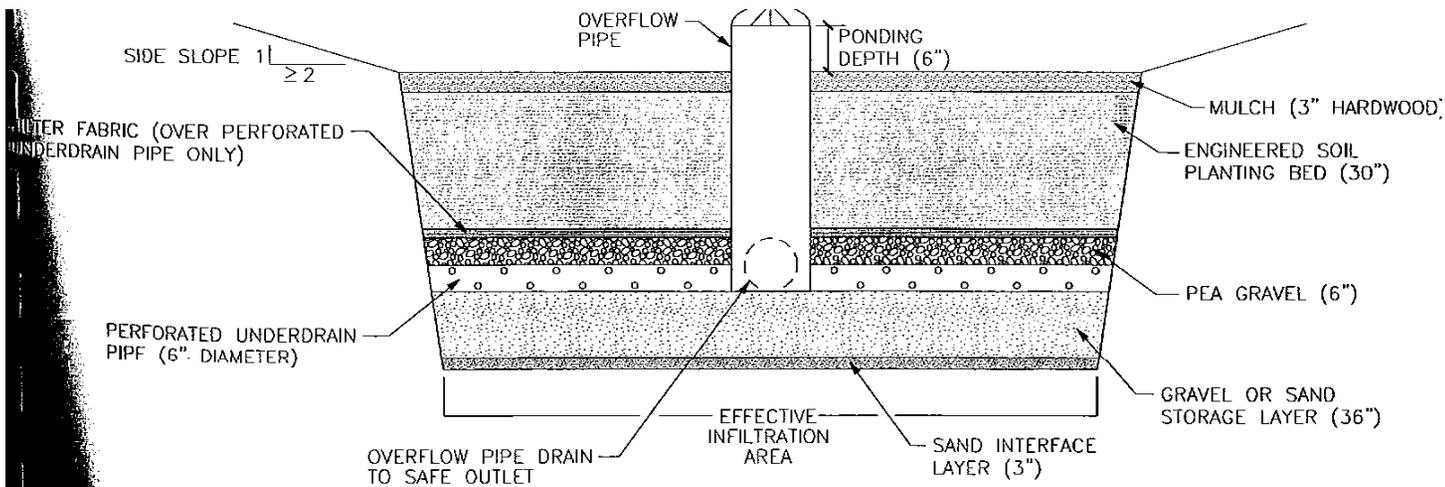
BIORETENTION DEVICE – CROSS SECTION ACROSS LENGTH OF DEVICE
