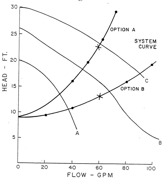
Fig. A-4 System performance curve and several pump performance curves for the example problem. For this example, the pump must provide a flow of at least 60 gpm
