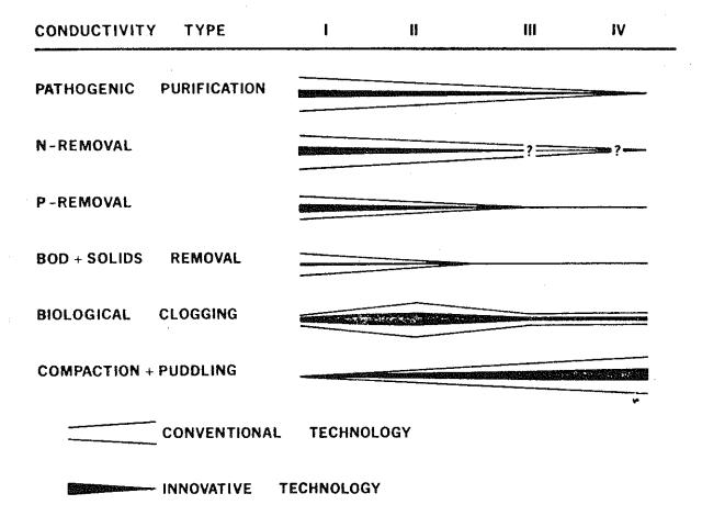
Fig. 2. Schematic diagram of different soils showing limitations(characterized as conductivity types) for achieving different processes of purification as a function of construction and management (technology) procedures. Potential limitations and problems increase as bands widen.
