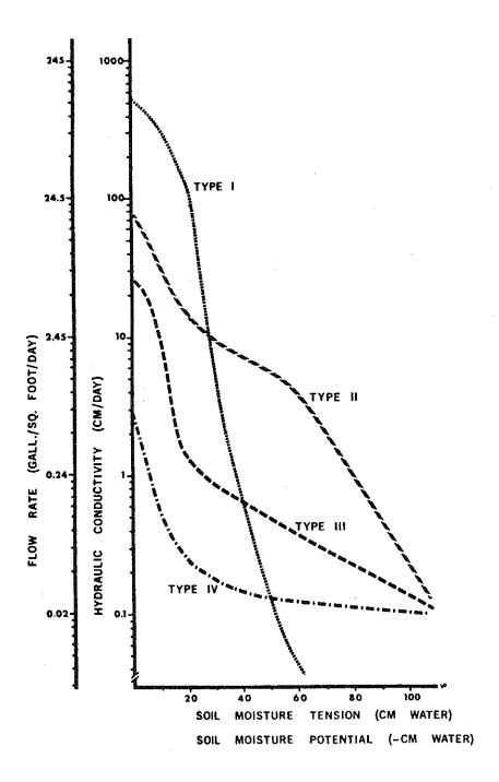
Fig. 1. Hydraulic conductivity (K) curves for four major types of soil (see text).
