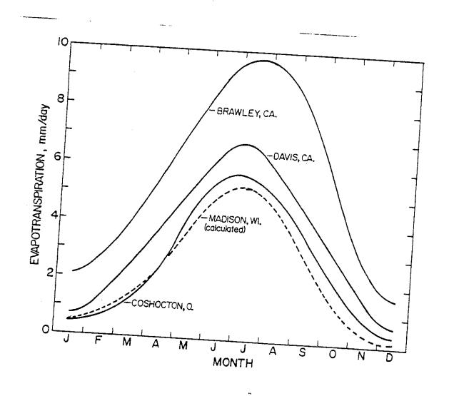
Fig. 1. Evapotranspiration from well-watered grass and alfalfa in lysimeters at different locations in the United States (from Jensen 1).
