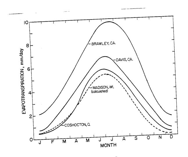
Fig. 1. Evapotranspiration from well-watered grass and alfalfa in lysimeters at different locations in the United States (from Jensen).
