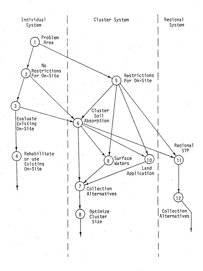
Figure 2. Facility Selection Procedure
