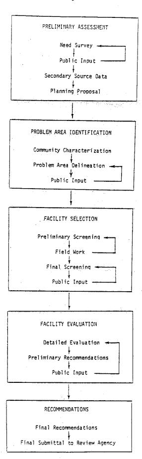
Figure 1. Wastewater Facilities Planning Procedure for Small Unsewered Communities
