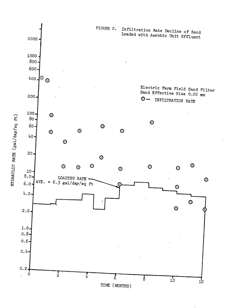
At this time, an accumulation of suspended solids on top of the sand had become 3/4 to 1-1/2 inches (1.9-3.8 cm) in depth. It is important to note that even at failure, the ultimate infiltration rate was  $\frac{>}{2}$  3.0 gal/day/sq ft (0.12 m/day).
