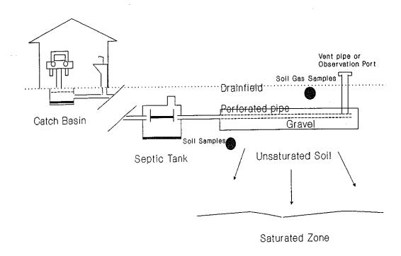
Figure 1. Approximate Location Where Soil and Soil Gas Samples Were Collected Beneath and Above Gravel Beds in MVSS Drainfields.
